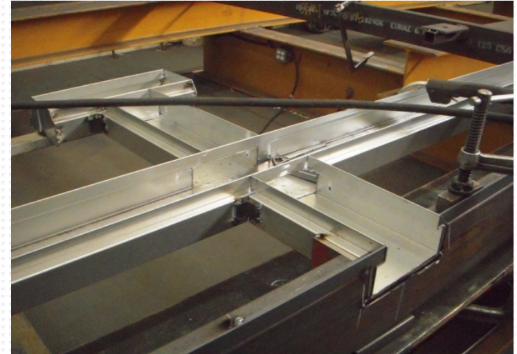
TYPICAL INTERSECTION OF 2 CHANNELS DURING FRAMING
