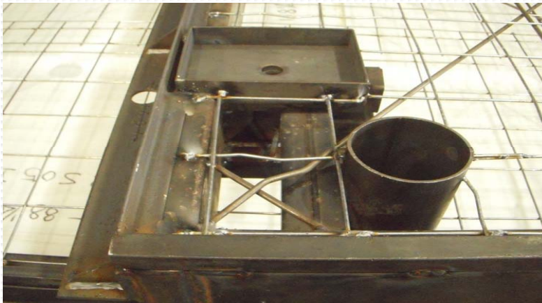
With plumbing sleeve pipes & double sided bracket connection
