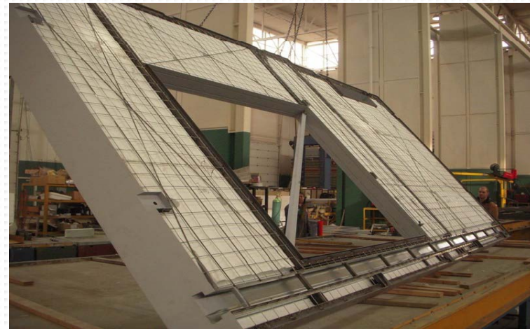
Placing the panel on its pallet in preparation for concreting
