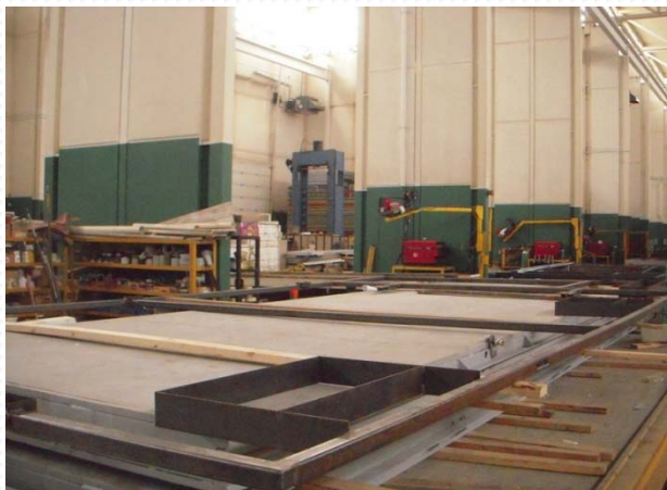
A typical 3.40 m x 10 m approx. interior panel with duct openings and very thin 2" x 2" x 1/8" HSS framing only
