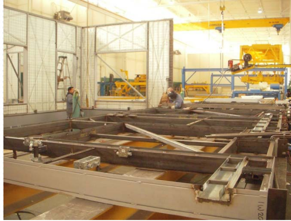
With the electric channels & temporary bracing in the central area of the main building
