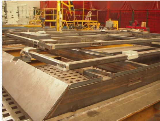
2" x 2" HSS framed panels stacked on top of mitred 8" thick panel & built-in electric channels.
