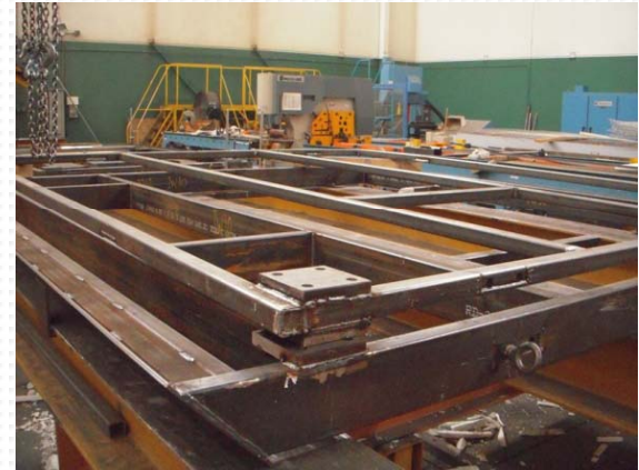
2" x 2" HSS framed panels stacked on top of mitred 8" thick panel & built-in electric channels.
