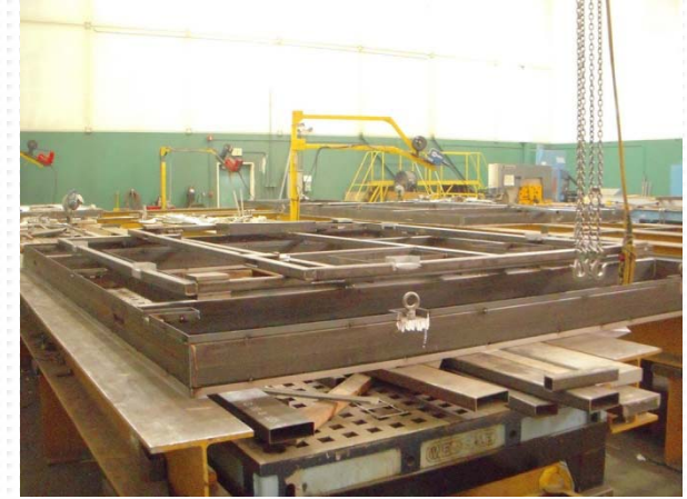
In the central East side of the main building showing 2" x 2" HSS frames
