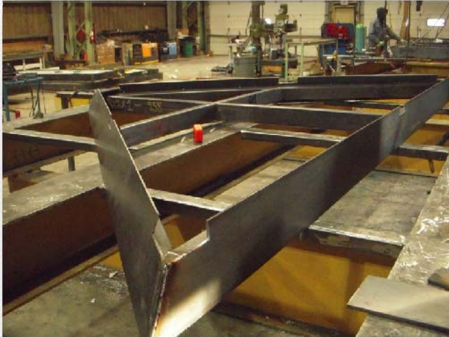
VARIOUS PITCHED ROOF PANELS UNDER FABRICATION
