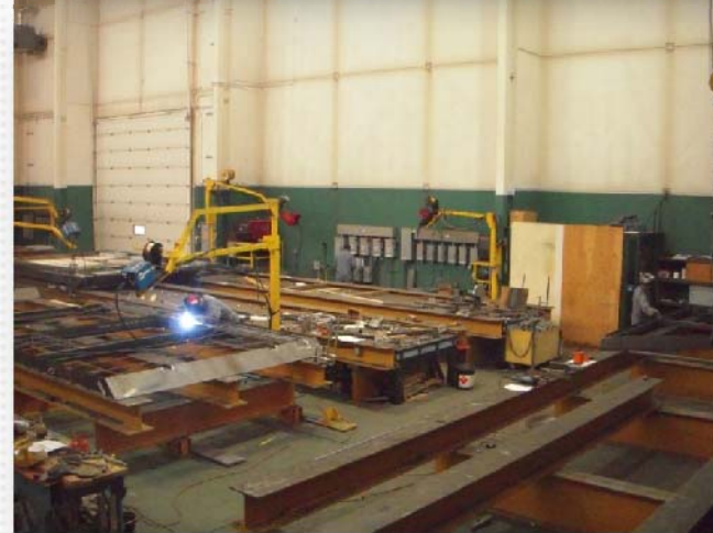
VARIOUS PITCHED ROOF PANELS UNDER FABRICATION
