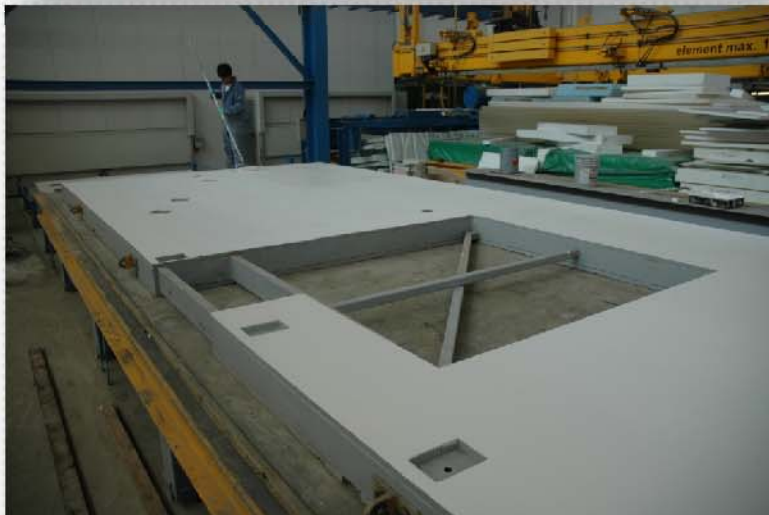
COATED PANELS READY TO BE BUNDLED TOGETHER IN 10-TON PALLETS
