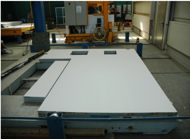
COATED PANELS READY TO BE BUNDLED TOGETHER IN 10-TON PALLETS INSIDE THE MANUFACTURING FACILITY
