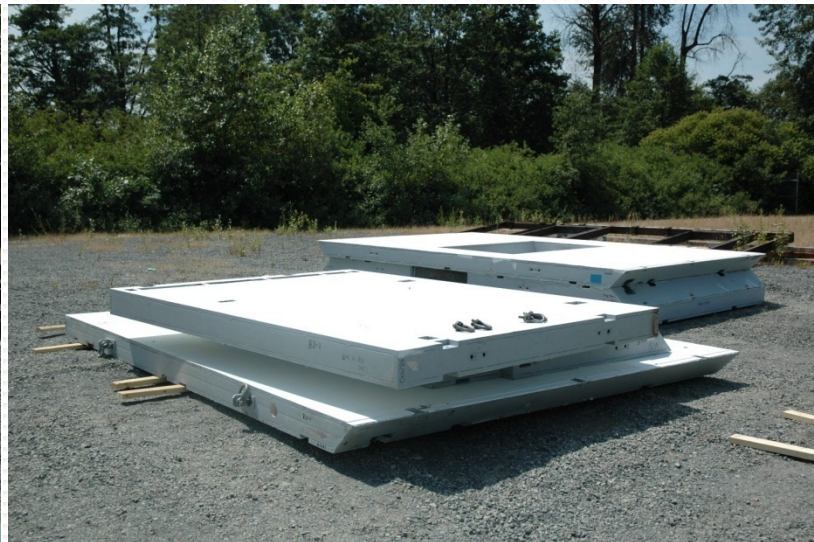
PANELS STAGED TOGETHER PRIOR TO PALLETIZING THEM INTO 10-TON BUNDLES OUTSIDE THE IHI R & D AND MANUFACTURING FACILITY
