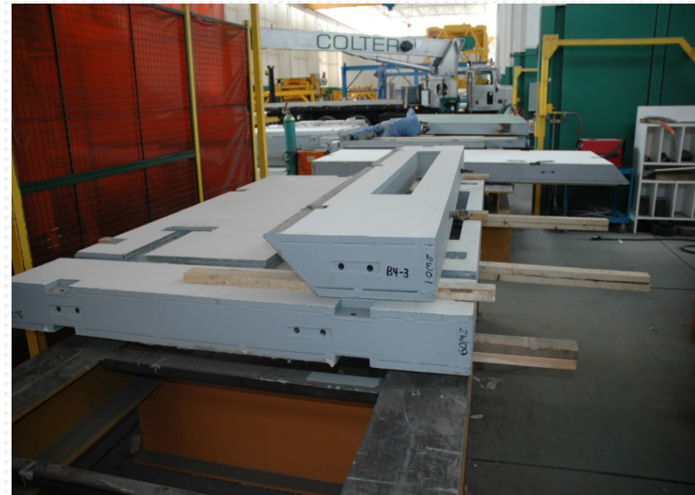
COATED PANELS READY TO BE BUNDLED TOGETHER IN 10-TON PALLETS INSIDE THE MANUFACTURING FACILITY
