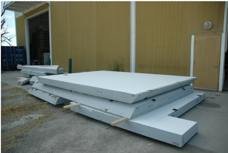
PANELS STAGED TOGETHER PRIOR TO PALLETIZING THEM INTO 10-TON BUNDLES
