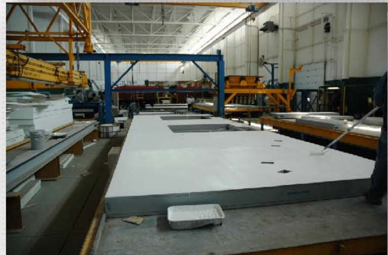
COATED PANELS READY TO BE BUNDLED TOGETHER IN 10-TON PALLETS
