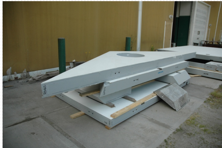
PANELS STAGED TOGETHER PRIOR TO PALLETIZING THEM INTO 10-TON BUNDLES
