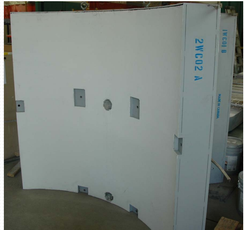
CURVED PANELS WITH CURVED STAINLESS STEEL TRIM BEFORE AND AFTER COATING
